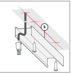
Pull secondary wires through ceiling & clearence in backbox.
