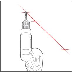
Drill all necessary powerfeed & pilot holes.
