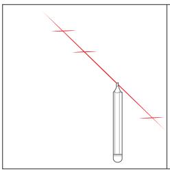
**4.** Project line using laser plumb and mark necessary mounting points using figure 1 as reference.
