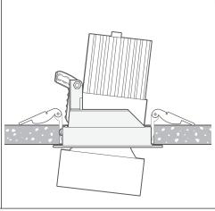
7. TO PAN & ROTATE Pull out only Select C mainbody(A) slightly so that reflector sits proud of surface.
