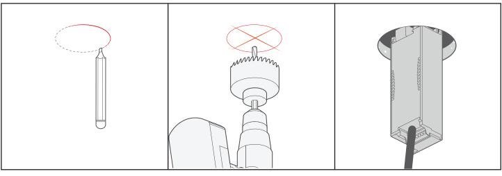
Measure and mark the appropriate placement of luminaire. Refer to figure A for critical dimensions.
