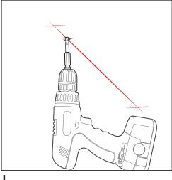
Using a plum laser, measure and mark position of light fitting. Drill Appropriate size hole for powerfeed.
