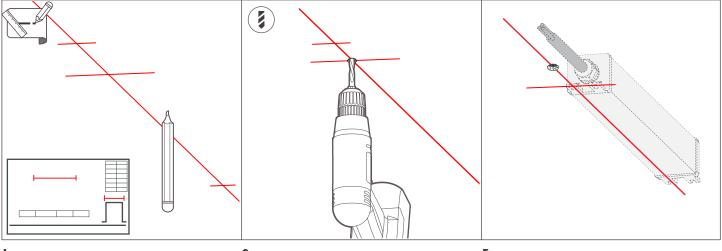
Project line using laser plumb and mark necessary mounting points using supplied Darkon drawing as reference.
