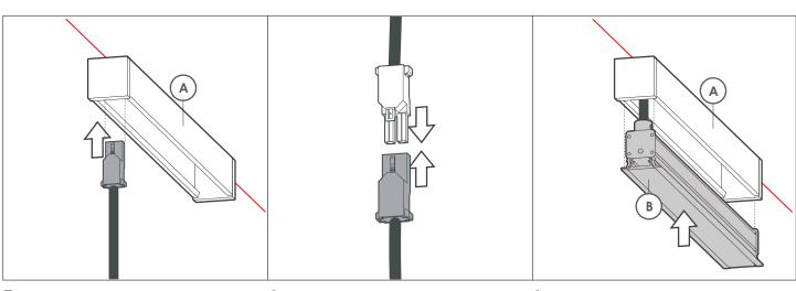
Insert plug through cutout of *Surfacebody(A)* Connect necessary plugs. and into previously drilled powerfeed hole in ceiling.
