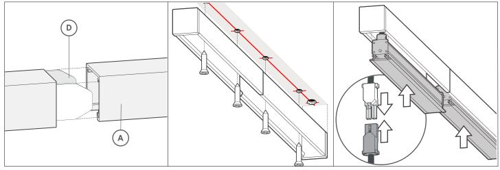
Align Linear Connector(D) of first Surfacebody(A) to sliding detail of second body.
