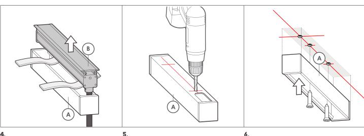
Remove Mainbody(B) from the Surfacebody(A). Remove supplied straps.
