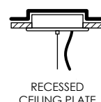
RECESSED CEILING PLATE CUT OUT Ø102mm
