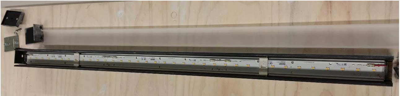
After IP5X dust test
