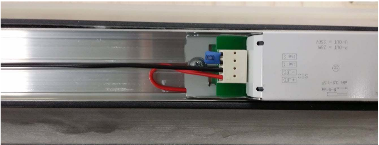
After IP5X dust test
