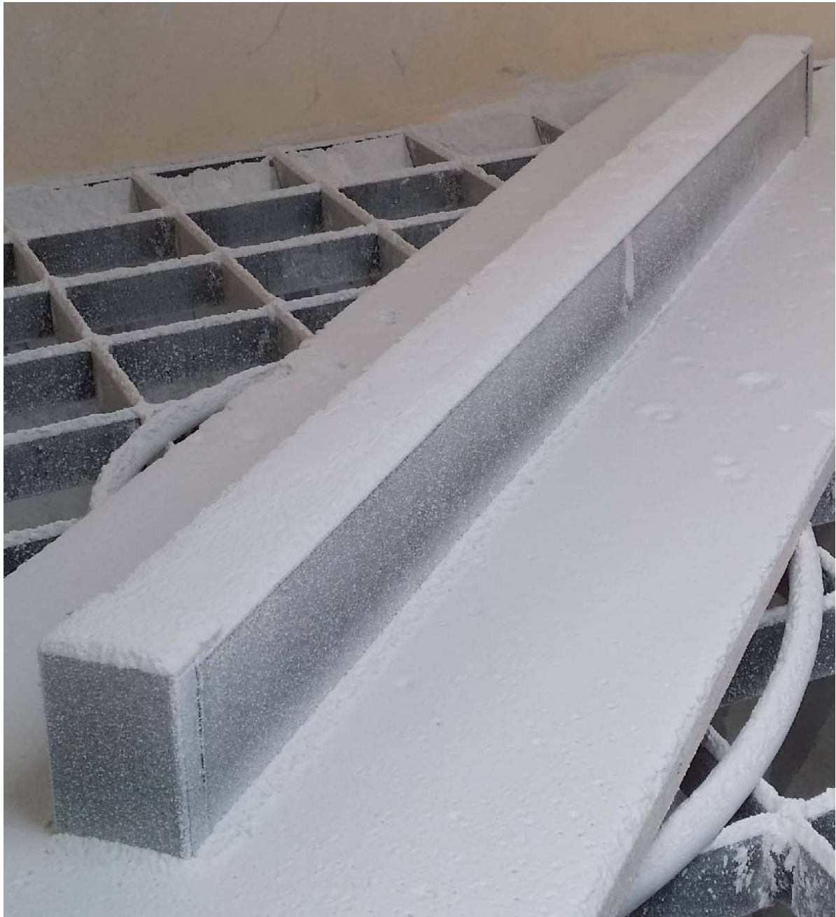
After IP5X dust test
