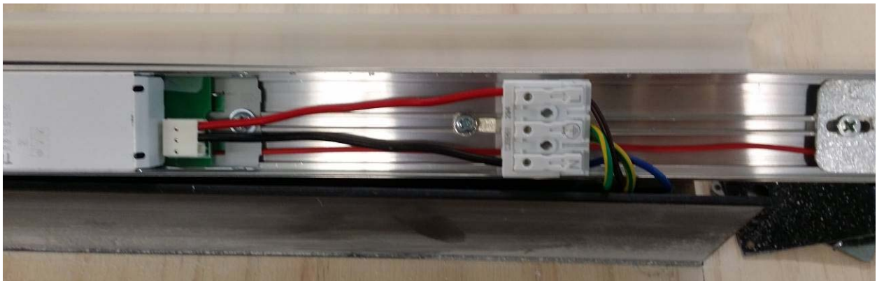
After IP5X dust test
