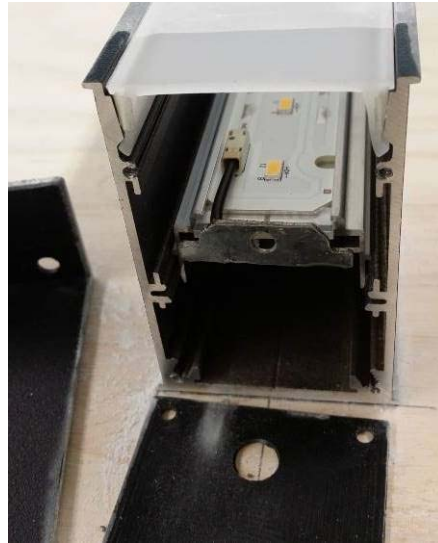
After IP5X dust test
