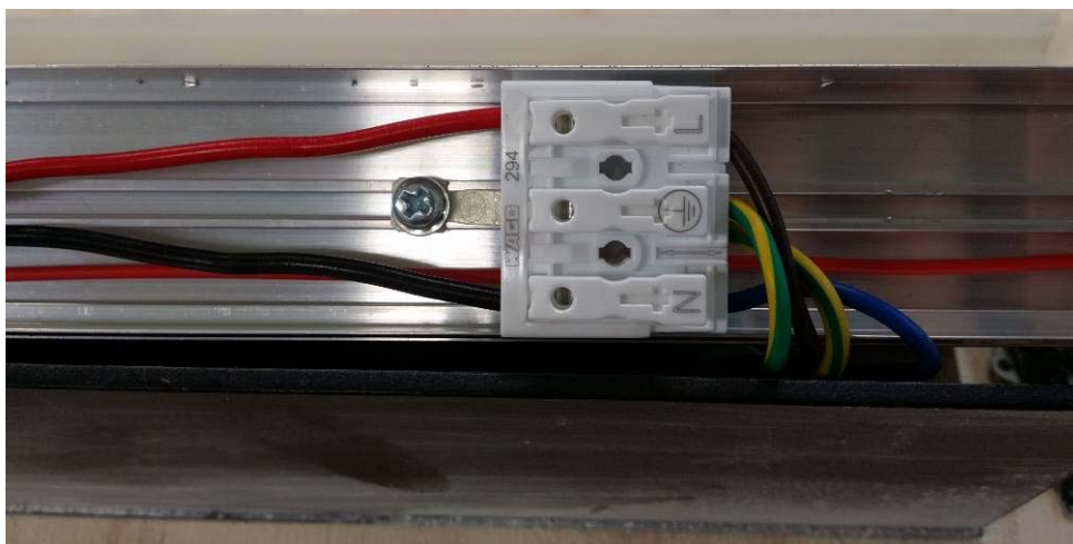
After IP5X dust test
