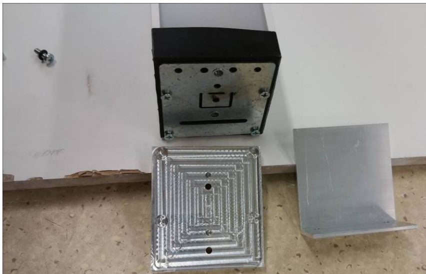
Figure 11: Post IP5X dust test
