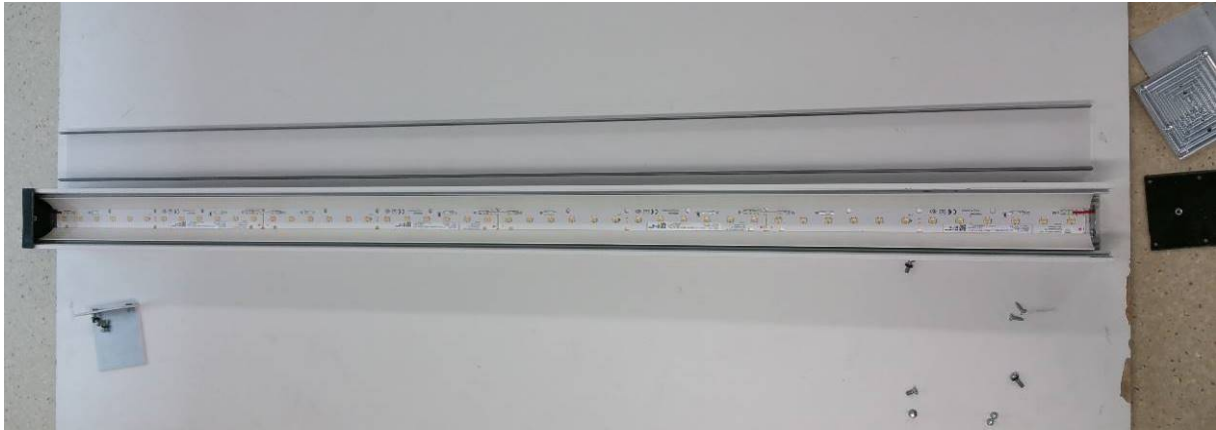
Figure 10: Post IP5X dust test
