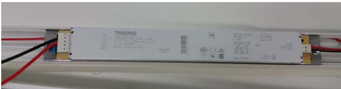
Figure 7: Post IPX5 water test
