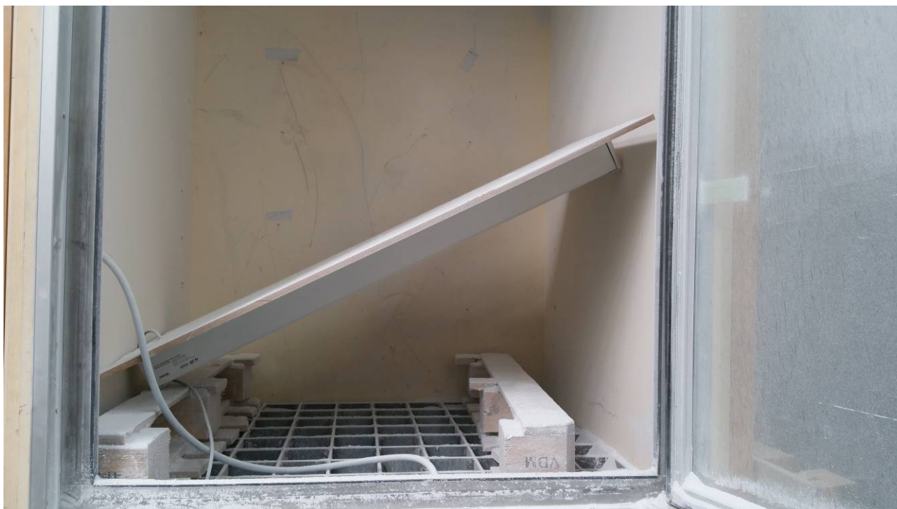
Figure 9: IP5X dust test setup
