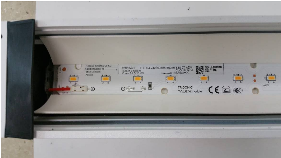
Figure 6: Post IPX5 water test
