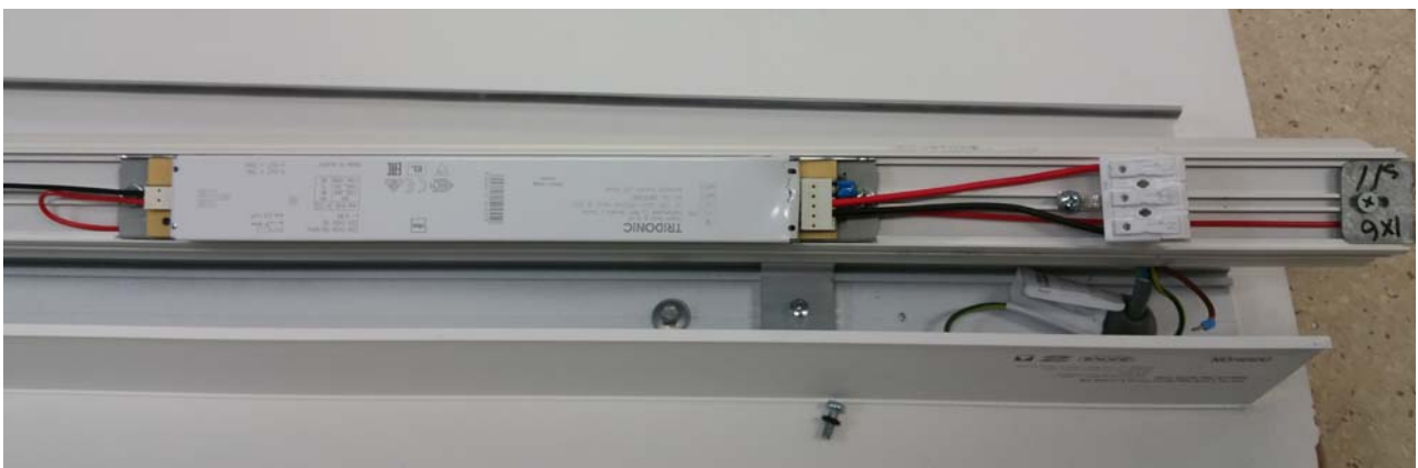
Figure 12: Post IP5X dust test
